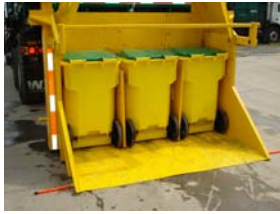
3-65 gallon toters in cart dumper
